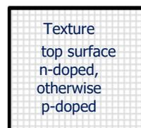
In a furnace, phosphoryl trichloride ( $\text{POCl}_3$ ) flows over the surface of the Si wafer at 900°C – 950°C. The [P] atoms penetrate the surface to a depth of ca. 0,2 µm. There, **the p-n junction** forms, which is important for the separation of charge in the solar cell.
