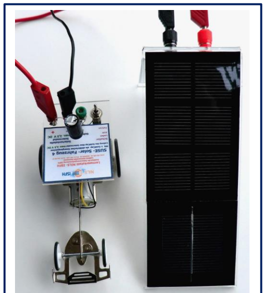
The solar vehicle 4 with the solar filling station (solar module) SUSE 4.34 (2.4V / 630 mA) Below the circuit board the solar electric motor is visible (with wires yellow/black)
