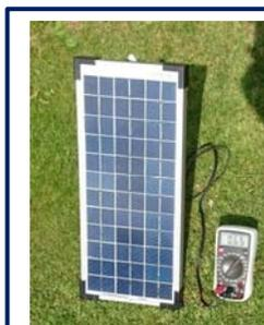
The **ammeter** shows the short-circuit current of 0.65 A.
