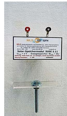
The technically identical device **SUSE 5.11** for stand systems with female connectors for 4mm lab wires
