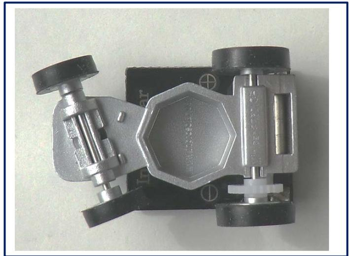
The **bottom side** of the solar mini racer: To the right of the rear axle in the cavity of the metal chassis a miniature electric motor is concealed, below the one-level gear is visible (white cogwheels), which drives the rear axle.
