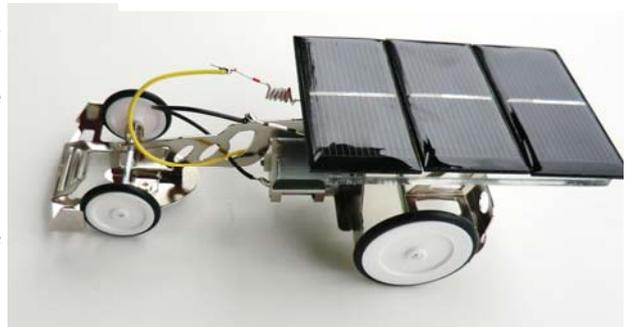
Afterwards the twisted wire connections are soldered up. The wire contacts must not touch each other! The photo shows the finished vehicle. In the end the transparent protective film is removed from the surface of the solar cells.
