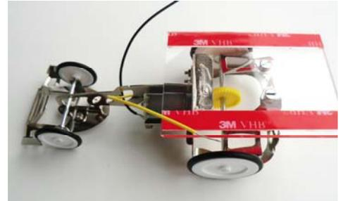
**Installation of the solar module:** Now the red protective film is removed carefully from both of the stripes of double-faced tape and the solar module is pressed carefully onto them, the width is identical, but the module overlaps in the front and the back by 5 mm. In driving direction the yellow wire should be up front. The yellow positive wire of the solar module is twisted with the yellow (positive) motor wire, the black module wire (negative) with the black motor wire (negative).
