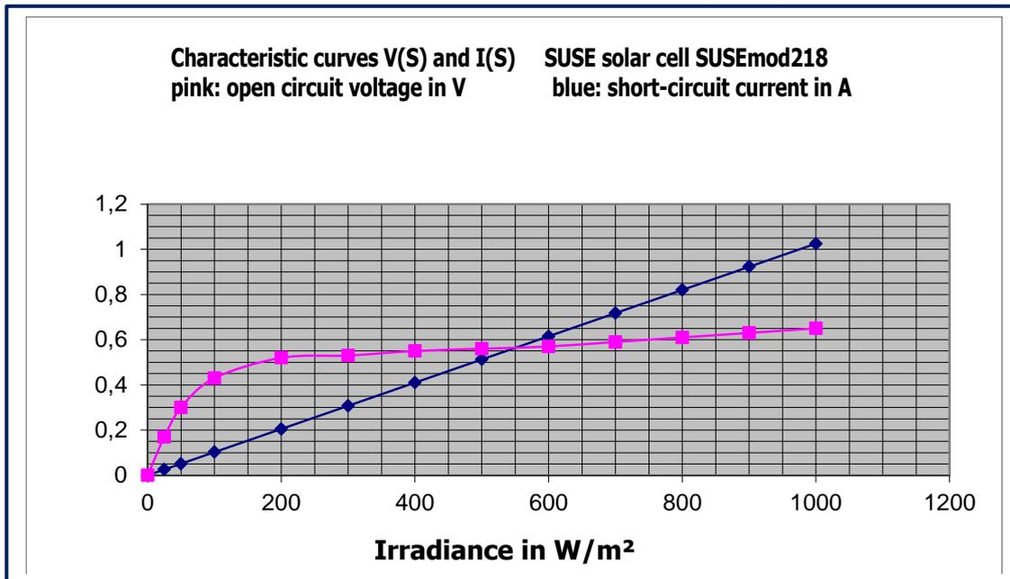
The **open circuit voltage  $V_{oc}$**  (exponential function!) is 0 in total darkness, increases strongly with small irradiances and then only slowly up to the maximum value of 0.64 V with 1000  $W/m^2$  (bright sunshine with blue sky, solar cell directed towards the sun).
