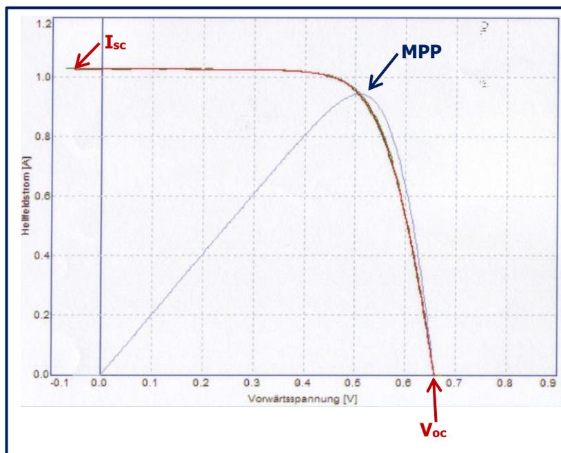
The **I-V characteristic curve** shows the dependence of the current on the voltage with a load of the solar cell in form a load resistor, with an irradiance of 1000  $W/m^2$  and a temperature of 25°C.
