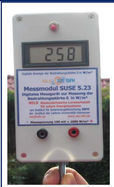
The measurement module SUSE 5.23 seen from the back side. At the top the operation switch is located, below the display for the display of the irradiance  $S$  in  $W/m^2$ .
