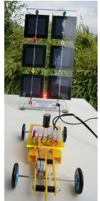
Charging of solar vehicle 2 with solar moduler SUSE 4.3RB (using 4 solar cells).
