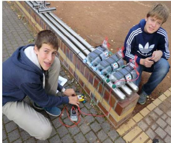
The two students charge the solar vehicle 1 with the solar cells of the solar boats. With the multimeter the charging process can be observed, the charging current or the voltage can be measured.
