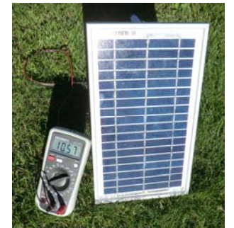
The open-circuit voltage in the sunlight: 10.57 V
