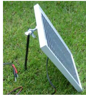
The adjustable positioner on the back side of the module
