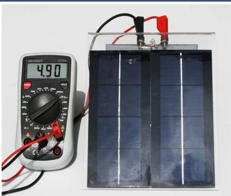
The solar module **SUSE 4.35** is a robust module with 2 solar modules SUSEmod6 with 8 solar cells in intern series connection. The **module voltage is 4.9 V**, the **short-circuit current 630 mA**, the **power 2.1 W** with standard testing conditions (irradiance 1000 W/m<sup>2</sup>, T = 25°C, AM 1.5).
