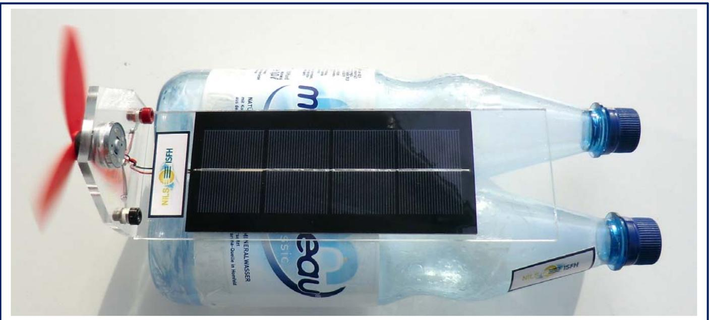
The solar boat 4 consists of a plexiglass base plate, which is bent to 90° at the site of the motor, there the solar electric motor, the test jacks and the big, red air-screw are located.
