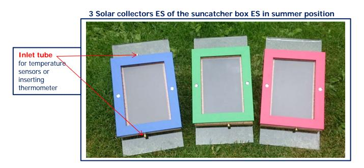
The solar collectors ES can be used for solar heat experiments in Primary School and in lower Secondary School.
