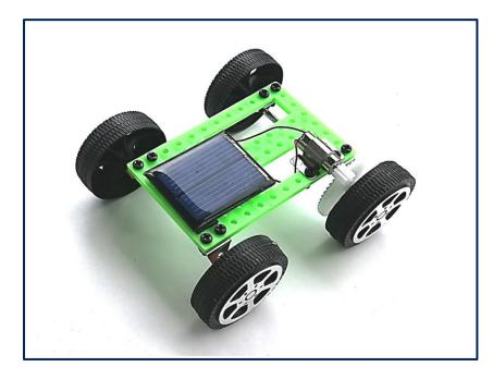
On the green chassis on the lefthand side, the little solar module is located, the two solar cells moulded within are clearly visible. With the 4 black screw pairs, 4 small metal brackets are mounted, the two axles run with low friction through 2 brackets each. At the end of both axles 4 synthetic wheels are attached.
