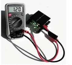
With a voltmeter, the module voltage, the short-circuit current, as well as the charging and discharging of the capacitor can be measured at the vehicle and measurement curves can be created. Here the measurement value of 1,20 V is shown during charging.
