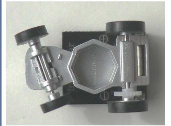
View of the solar mini racer: **On top** of the metal chassis the small solar cell is visible, on the right the wheels of the rear axle, on the left the steerable wheels of the front axle.
