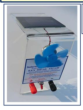
Also multiple devices SUSE CM4MSB can be connected in series. With 6 devices in series connection e.g. a 3 V radio (e.g. SUSE solar radio 4.36) or LEDs in all colors (SUSE 4.15) can be operated in the daylight.
