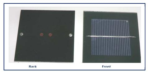
Below the laminated and encapsulated surface the actual solar cell 52 x 52 mm is visible.
