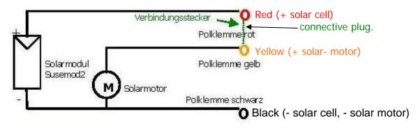
The solar module Susemod2 consists of 1 solar cell that is embedded robustly and break-proof. At a solar irradiation of 1000 W/m² (bright sunshine with deep blue sky) the open-circuit voltage is 0.6 V, the short circuit current 900 mA. The solar motor can be seperated or connected through the connective plug.
