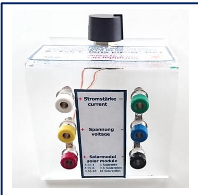
The solar load module SUSE 4.55 Top: General view from the top Bottom: Front side with the 3 socket pairs, on the top side the turning knob of the potentiometer is visible.
