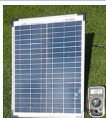
The **amperemeter** shows the short-circuit current of 1.27 A.
