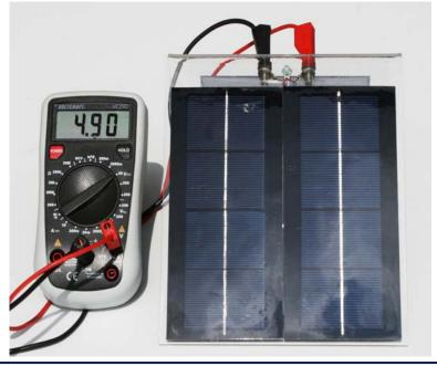
**Top:** The solar module SUSE 4.35, on the front there are 2 modules SUSEmod6, on the back the 2 jacks red (+) and black (-), in between the green LED as operation display, are visible. The voltmeter shows the module voltage of 4.9 V.
