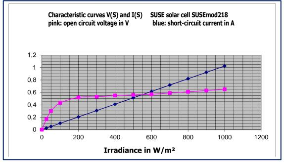
The **open circuit voltage V**<sub>oc</sub> (exponential function!) is 0 in total darkness, increases strongly with small irradiances and then only slowly up to the maximum value of 0.64 V with 1000 W/m<sup>2</sup> (bright sunshine with blue sky, solar cell directed towards the sun).
