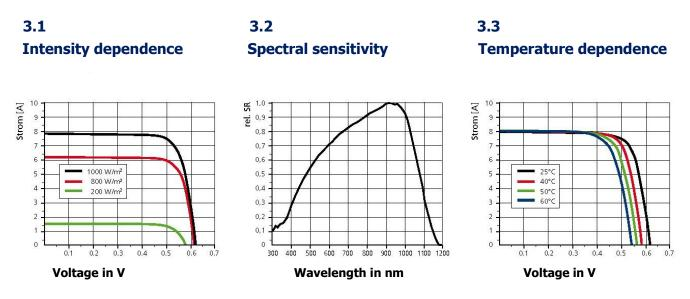
The graph on the left hand side 3.1 shows the intensity dependence of the I(V) characteristic curves dependent on the irradiance S of the irradiated light. (1000 W/m<sup>2</sup> is equivalent to bright sunshine in the sumer with a blue, cloudless sky, 0 W/m<sup>2</sup> is total darkness).
