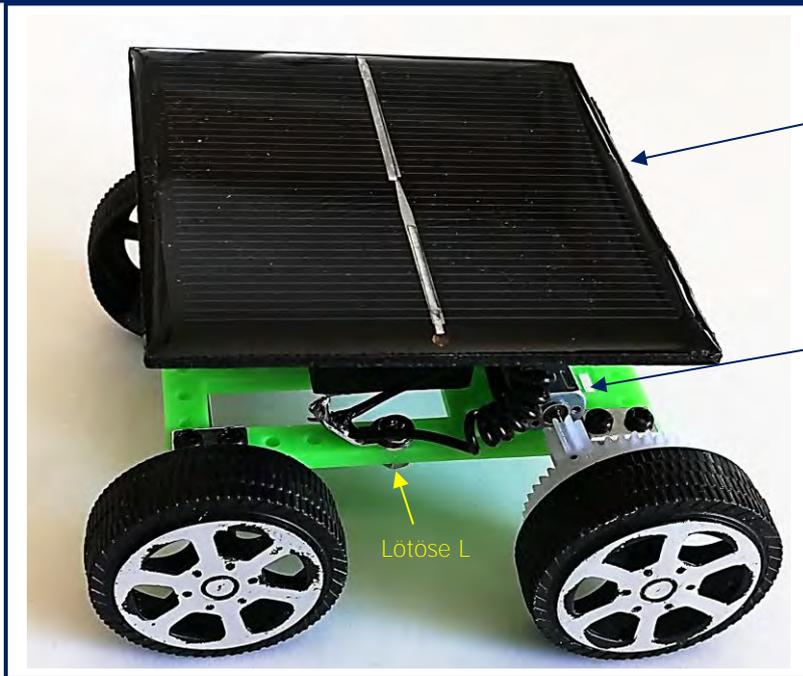
Solarmodul 60mm x 60mm
