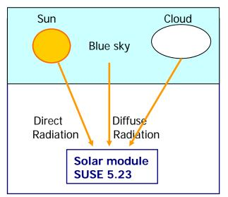
Fig.3: Global radiation = sum of direct and diffuse radiation
