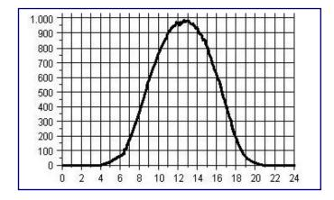
Fig.5: Intraday progress of an irradiance in  $W/m^2$  (y-axis) from 0 to 24 o'clock (x-axis) on a cloudless summer day (source: NILS- ISFH). The measurement module **SUSE 5.23** is mounted on a southerly roof with 35° inclination.
