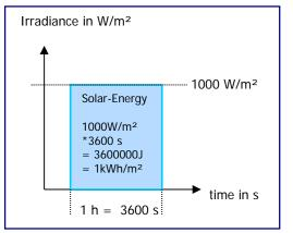
Fig.4: Irradiated solar energy with an irradiance of 1000 W/m<sup>2</sup> and a time span of 1 h = 3600 s
