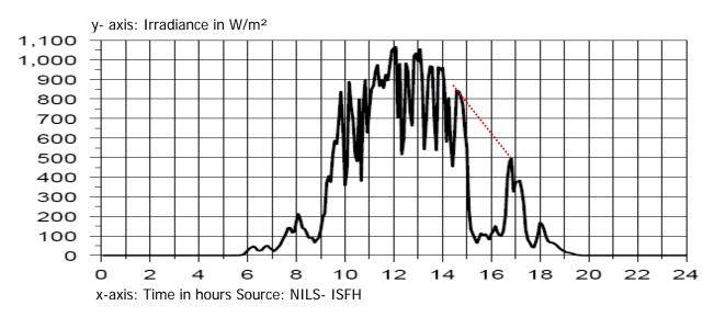
**Recording of a day profile of the irradiance and determination of the irradiated energy** The cavings of the irradiance caused by clouding are clearly recognizable, this happened several
