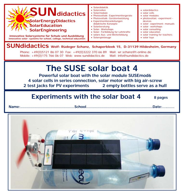
The solar boat 4 consists of a plexiglass base plate, which is bent to 90° at the site of the motor, there the solar electric motor, the test jacks and the big, red air-screw are located.
