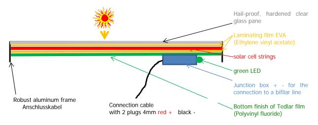
Soldered in the junction box of the solar module SUSE 4.51 is a 1.5 m long bifilar connection cable with two 4 mm bunch plugs red (positive) and black (negative), a green LED shows operational readiness.
